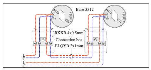
Example showing how to connect the Analog base 3312.
